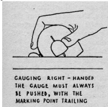
Checking measurement of the marking gauge
